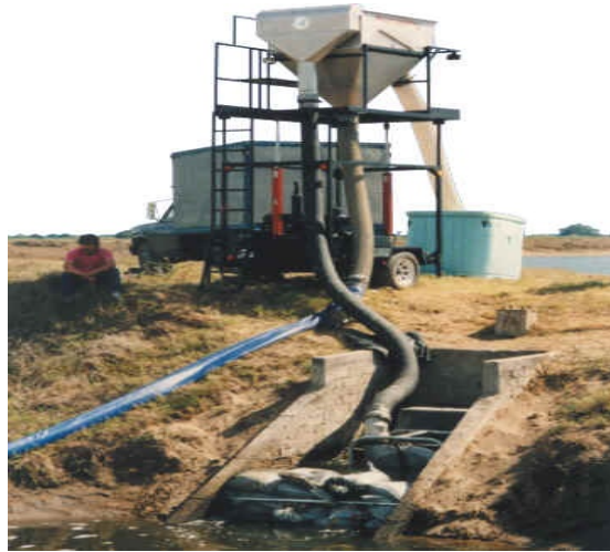
Figure: Cavity Pump Harvester, different models with varying harvesting capacity per hour
